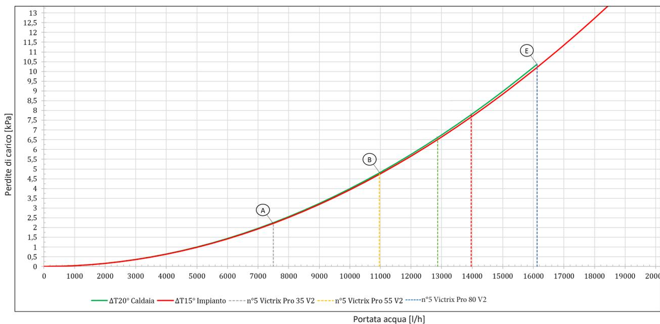
—  $\Delta T20^\circ$  Caldaia / Boiler —  $\Delta T15^\circ$  Impianto / System
