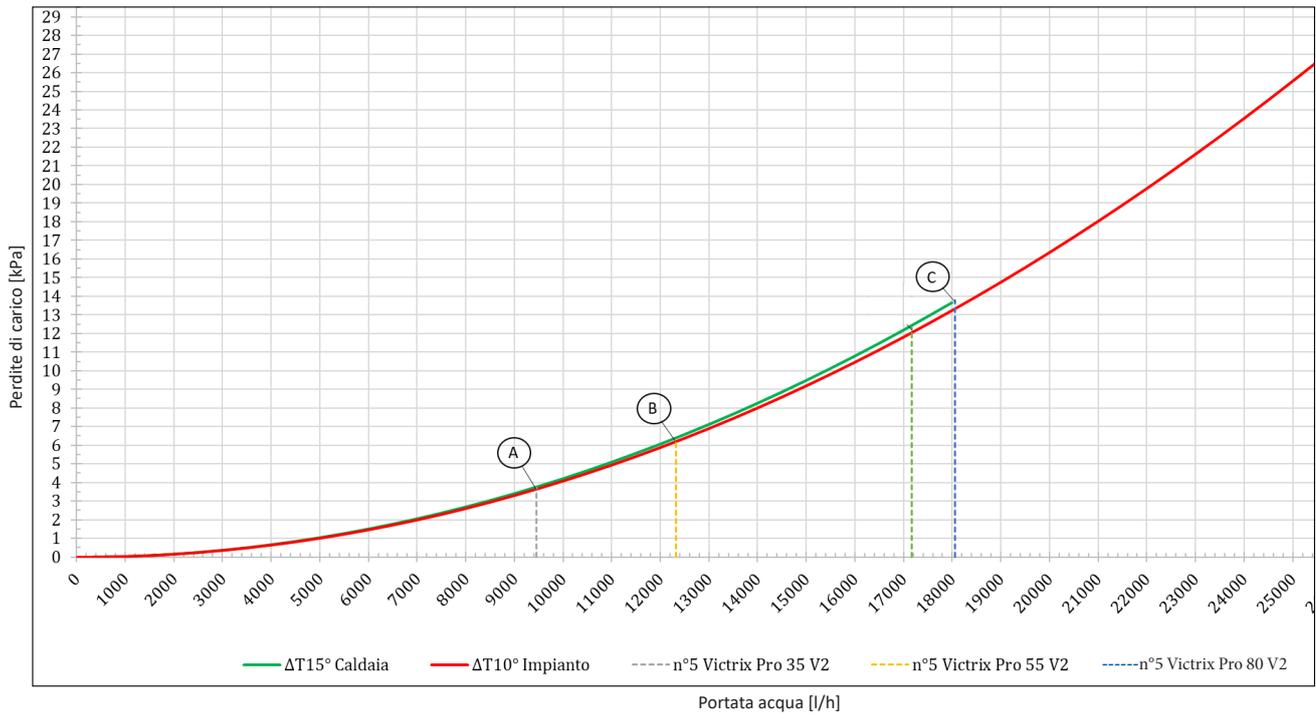
—  $\Delta T 15^\circ$  Caldaia / Boiler —  $\Delta T 10^\circ$  Impianto / System
